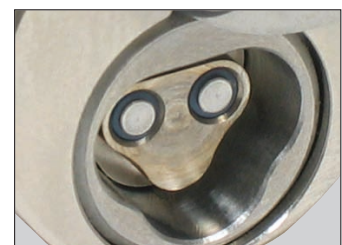
Figure 4: Stainless steel lock face with two contact points
