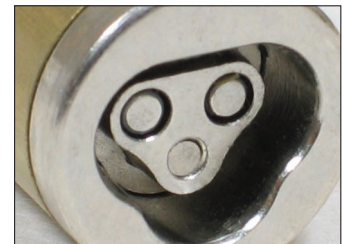
Figure 2: Nickel-plating on lock face with three contact points
