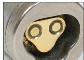
Figure 5: Lock in Figure 1 after cleaning dirty nose and contacts
